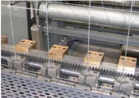
*The line and tie wires are fed from wire carriers positioned under the back frame at the rear of the machine.*
