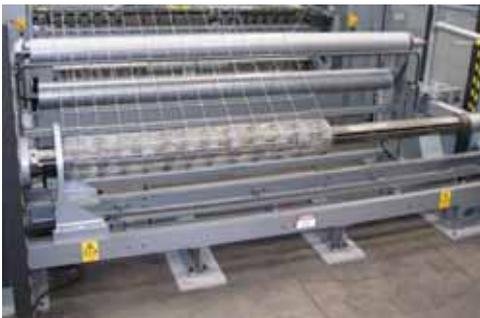
*The finished fence is wound onto a slotted mandrel. The take-up system has a variety of settings to accommodate different fence specifications and roll lengths. The completed roll is then stripped mechanically.*
